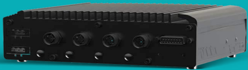
CN7000 example Milspec - Fanless, ruggedised IP67 form factor.
